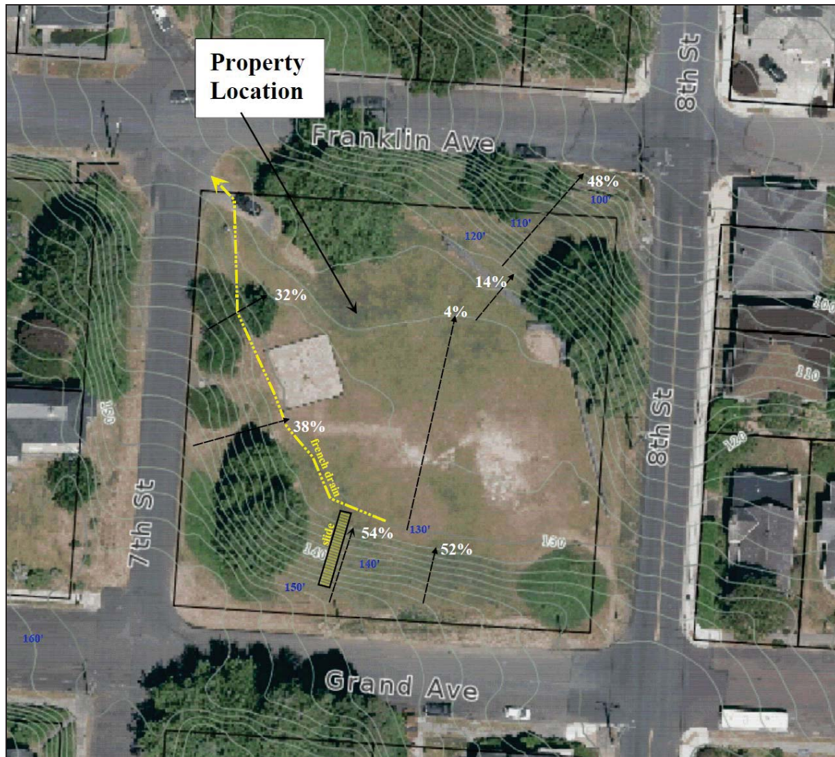
Figure 3: Aerial view of TL 7300 with 2 ft topographic contours and the position of the proposed slide and French drain line shown. The position of the route is approximate; it has been borrowed from drawings provided by the Friends. The route may need to deviate to avoid damaging tree roots or to permit easy construction and grading of the drain. The drain extends about 15 ft east of the toe of the slide in order to soak up any accumulating storm water near the base of the project. Downslope direction is indicated by arrows, inclinations expressed in percents, calculated from the rise and run; the lot is 200 ft on a side. See Figure 4 for construction details.
